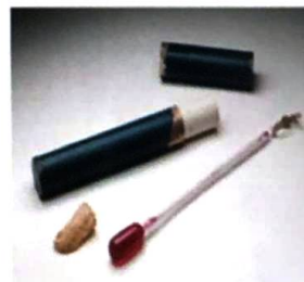
Red bulb and piece of cloth : kata thermometer.
